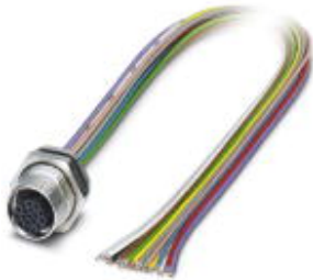
Sensor/actuator flush-type socket, 17-pos., M12 SPEEDCON, rear/screw mounting with Pg9 thread, with 0.5 m halogen-free TPE litz wire, 17 x 0.14 mm
